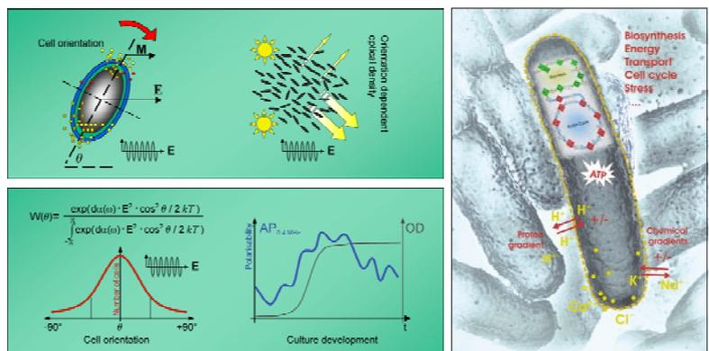
This in turn leads to a minuscule force effecting each cell to slightly change its spatial orientation within the suspension flow. This change in orientation correlates directly with the free ion concentration in the cytoplasm and is being picked up extremely sensitively and precisely by our proprietary high-end photometric sensors.
